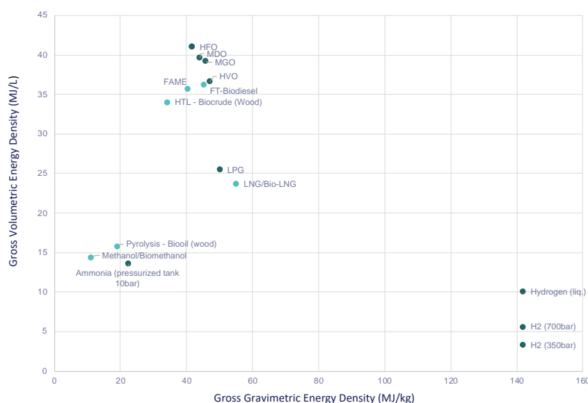
Figure 2: Gross gravimetric and volumetric energy densities of biofuels (light blue) and other existing and potential marine fuels (dark green). Calculations are based on values from Pedersen et al., 2016; Mohan et al., 2006; Zamfirescu & Dincer, 2009; NIST, n.d. The values for compressed hydrogen and ammonia have been calculated under ambient temperature conditions. N.B. Lignin fuels are not included as data on energy densities are not currently publicly available.
