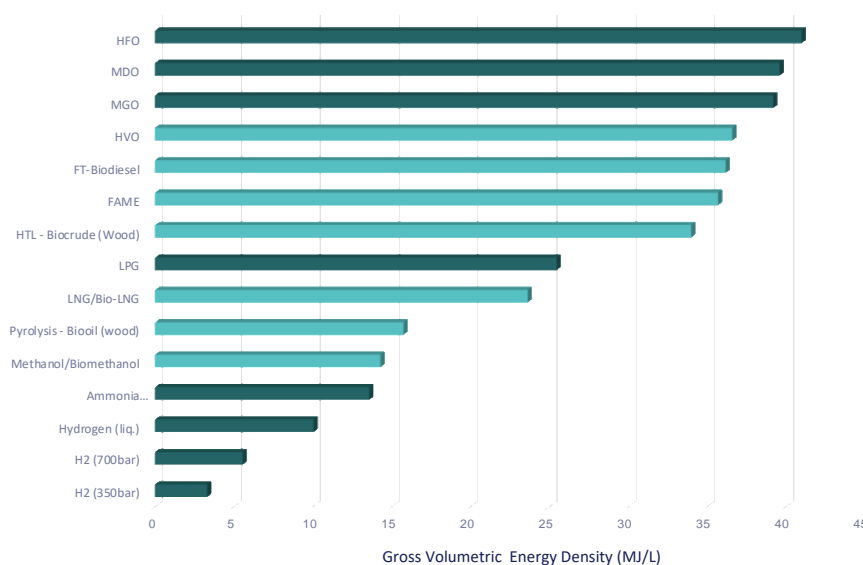
Figure 3: Gross volumetric energy densities of biofuels (light blue) and other existing and potential marine fuels (dark green). Calculations are based on values from Pedersen et al., 2016; Mohan et al., 2006; Zamfirescu & Dincer, 2009; NIST, n.d. The values for compressed hydrogen and ammonia have been calculated under ambient temperature conditions. N.B. Lignin fuels are not included as data on energy densities are not currently publicly available.
